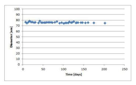
A graph depicting the diameter of PEG-coated silica nanoparticles measured using the Dynamic Light Scattering (DLS) technique during a period of over 200 days, is shown. The size deviation of the nanoparticles is within the limits of +/- 2 nm.
